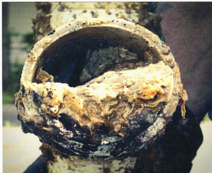
The sewer pipe (above) is blocked by grease buildup.
